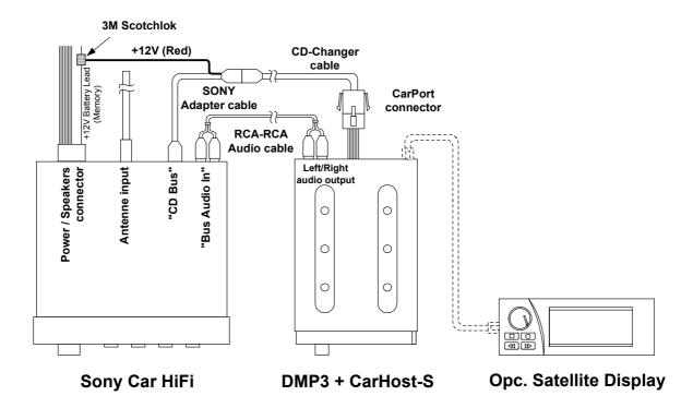
This diagram shows the installation with a SONY car radio. Usage of CarHost-A developed for ALPINE MBUS head units are similar. Please note that the exact wiring configuration will be determined by the CD Changer Adaptor necessary to support your car radio. The documentation included with the CD Changer Adaptor will provide an exact schematic for your vehicle.
