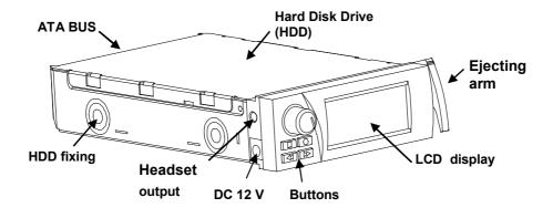
If you purchased a **DMR3** in order to fit your own hard disk, the first step is to install and format the disk using the standard WINDOWS tools. The **DMR3** is connected to the PC via the internal IDE PC docking bay.
