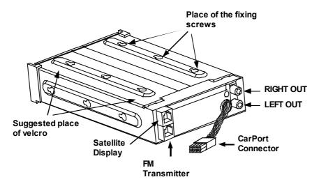
If you install the CarHost frame with the supplied screws, first mark the required location of the screw holes, taking care to avoid key parts of the car such as the fuel line or braking system, then carefully drill the holes and screw the car frame into position.
